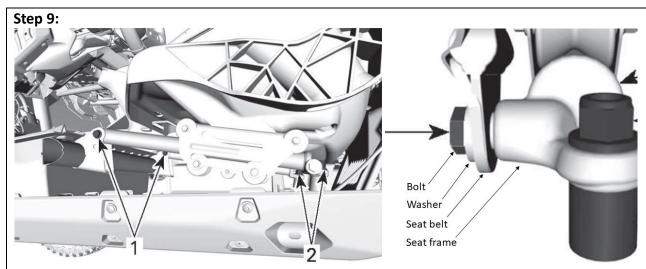
Replace the driver seat. Tighten the rear nuts (2) to 48ft-lbs and the front nut and bolts (1) to 18 ft-lbs.
