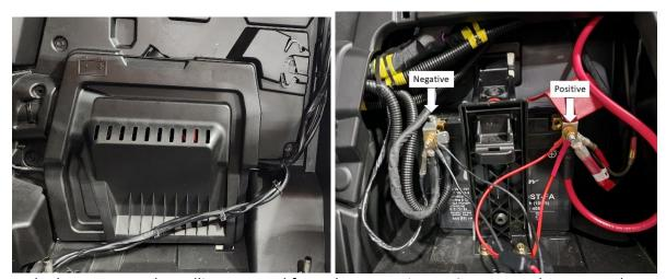
Remove the battery cover by pulling outward from the top. Using a 10mm wrench, remove the negative battery cable followed by the positive.
