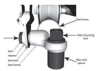
Using a 5/8 socket, remove the driver side seat belt bolt securing the coiled cable and seat belt to the seat.
