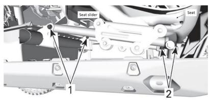
To remove the front seat, use a 13mm wrench and socket to remove the front bolts (1). Use a 18mm socket to remove the rear seat nuts (2) from the studs. Lift the seat up and out to remove.
