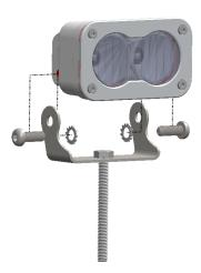
Place the M6 flange bolt through the universal bracket and attach the bracket to the S2 using the included parts bag.
