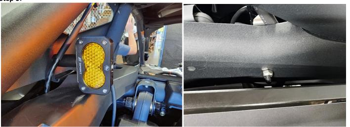
Place the 1.75" spacer on the M6 bolt and slide the bolt through the B-Pillar. Secure it with the ¼" washer and M6 nylock nut. Tighten using the 10mm wrench and socket.
